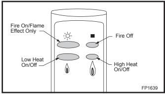
Fig. 5 Remote control handset.
